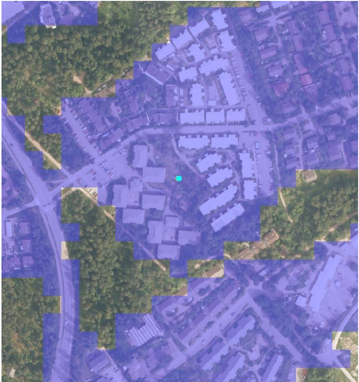
Figure 4. Green areas (forest) >MMU amongst and in the edges of buildings are incorrectly included in the HRL built-up (purple). Scale 1:2000, coordinates E: 377150, N: 6678950.
